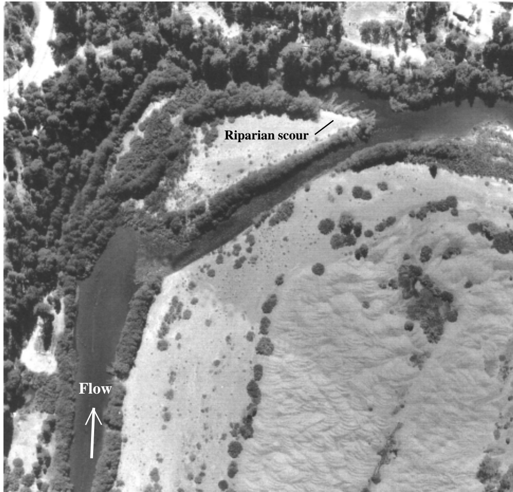
Figure 2.10 Gold Bar (RM 106.3) alluvial deposit in 1975. Note the riparian scour effects of the 1974 flood (14,000 cfs) along the downstream edge of the point bar. Discharge = 213 cfs, scale approximately 1" = 225'.
