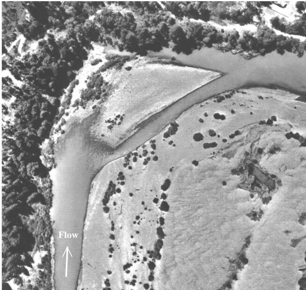
Figure 2.8 Gold Bar (RM 106.3) alluvial deposit in 1961. Note absence of vegetation along the channel edges and scoured dredger tailings along the inside of the bend. Discharge = 192 cfs, scale approximately 1" = 225'.
