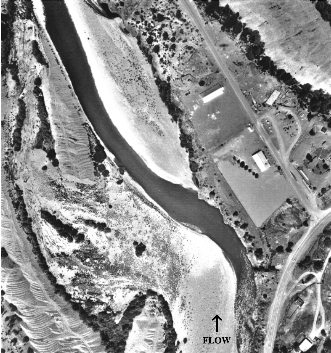
Figure 2.15 Pre-TRD alternate bar unit on the Trinity River near Junction City (RM 80.0), 1961 photograph. Lewiston discharge = 192 cfs, scale approximately 1" = 200'.
