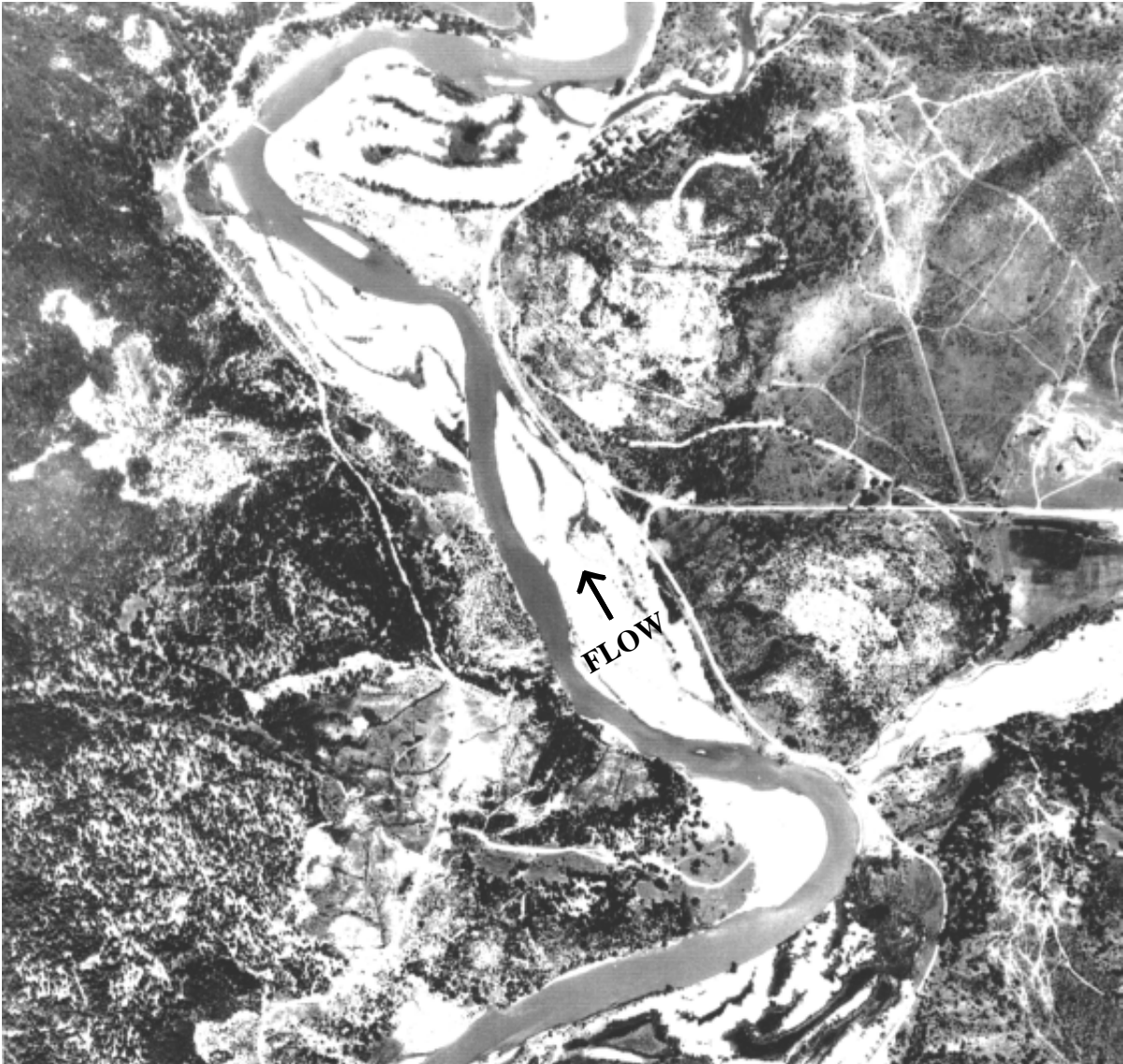
Figure 2.17 Alternate bar sequences and floodplains near Junction City in 1960. Lewiston discharge = 5,000 cfs, scale approximately 1" = 1,150'.
